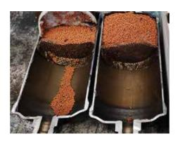
In a non-original filter, the amount of filler takes **less than 1/3 of the filter's volume.** This significantly reduces its capacity to remove moisture and other harmful impurities.
