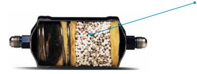
Some non-original dehydrators use a granular filler. The filler granules rub against each other during vibration or during refrigerant passage, thus causing the risk of fine particles entering into the system
