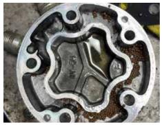
The use of **non-original filters** can lead to the entry of filler particles into the system and the subsequent **blockage** and **malfunction** of the system elements, up to the **breakdown** of the compressor.
