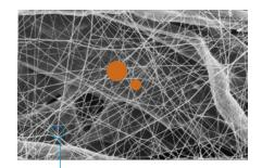
The fibers in the Thermo King filter media have submicron diameter and small interfiber spaces, which result in more contaminant being captured on the surface of the media and lower restriction.
