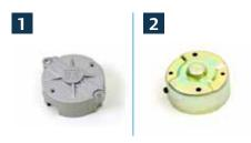
Thermo King starters use a cast aluminum end cap instead of the stamped, zinc-plated steel end cap used by various competitors. Aluminum holds up better to corrosion, and the cast machining process provides a stronger, more durable design that is important for high vibration applications.
