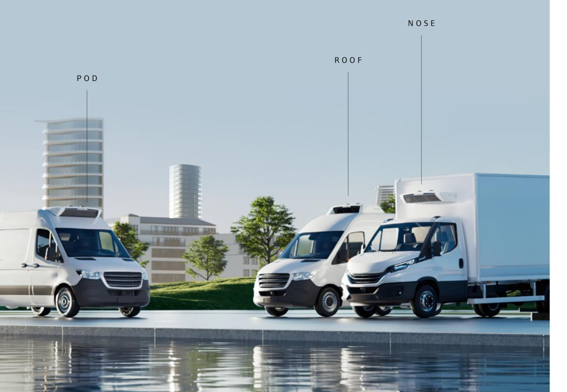
HIGHER DAILY PAYLOADS Not only is the E-Series extremely compact, but it is also extremely light - about 50% lighter than legacy units. That means less weight and more cargo **space** with each delivery cycle.
