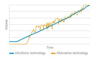
Compared to alternative fuel level sensor technologies, the UltraSonic Fuel Sensor provides the most accurate fuel level, no matter how full the tank is.
