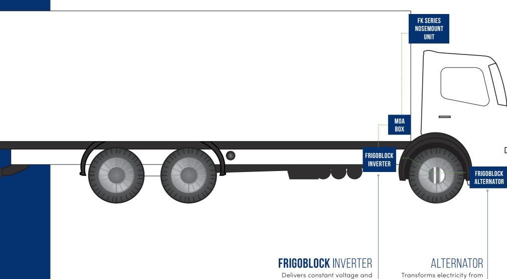
frequency to the unit regardless of vehicle engine speed. Guarantees rapid start-up of the unit with low mechanical stress. Provides optimum load temperature control with minimum power consumption.
