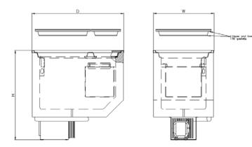
The CRUISE 40 CUBIC can also be installed as a built-in top opening cooler box.
