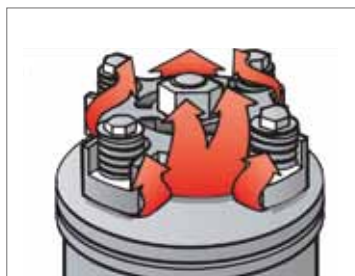
Under abnormal conditions, when extreme pressure is created by liquid refrigerant or oil entering the cylinder, the entire discharge valve cage lifts to vent the excessive pressure. This 2-stage pressure relief system helps extend overall compressor life.
