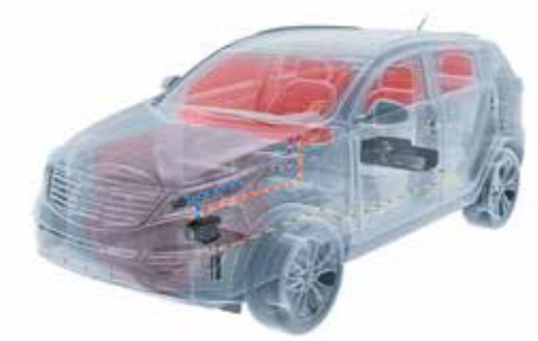
Fuel Operated Water Heater
