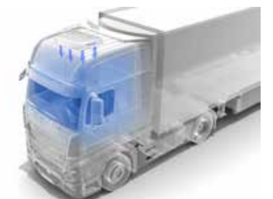
Parking Air-conditioning system
